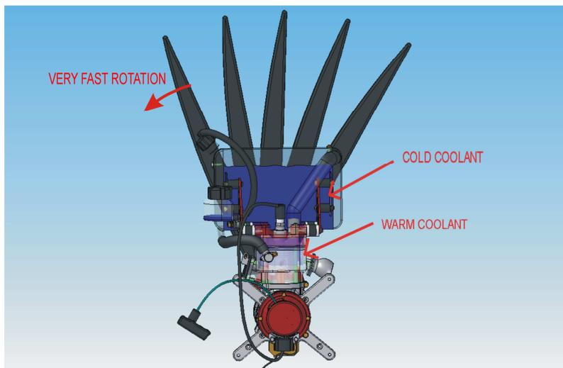
The fast rotation of the helix (high RPM as around 10000), cools the radiator and doesn't allow to coolant to circulate.
