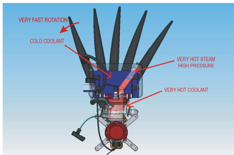
At the end, the very hot steam, can't push cold water into radiator and coolant doesn't begin circulating.
