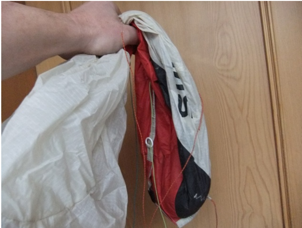
Picture 1: Right hand stabiliser of the accident glider containing approx. 1,5 kg sand.
