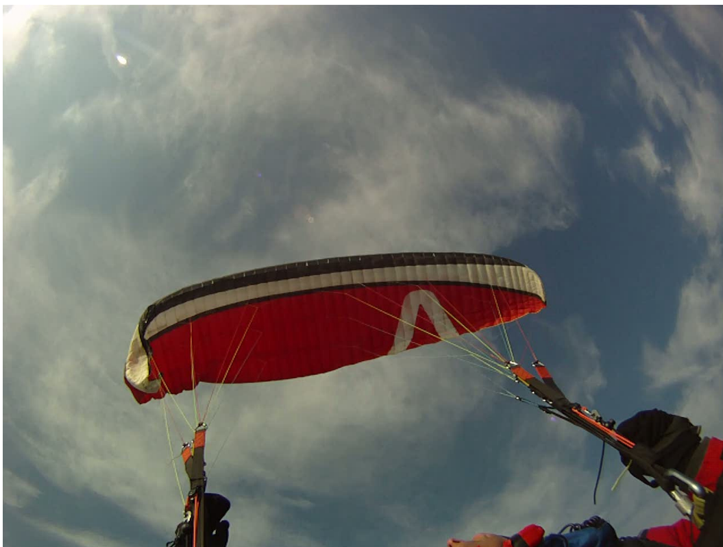
Picture 4: Cravat on the right hand stabiliser, the glider rapidly turns to the right.
