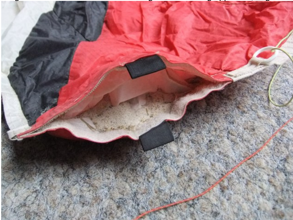
Picture 2: The sand could have been easily removed via the Velcro opening on the glider.
