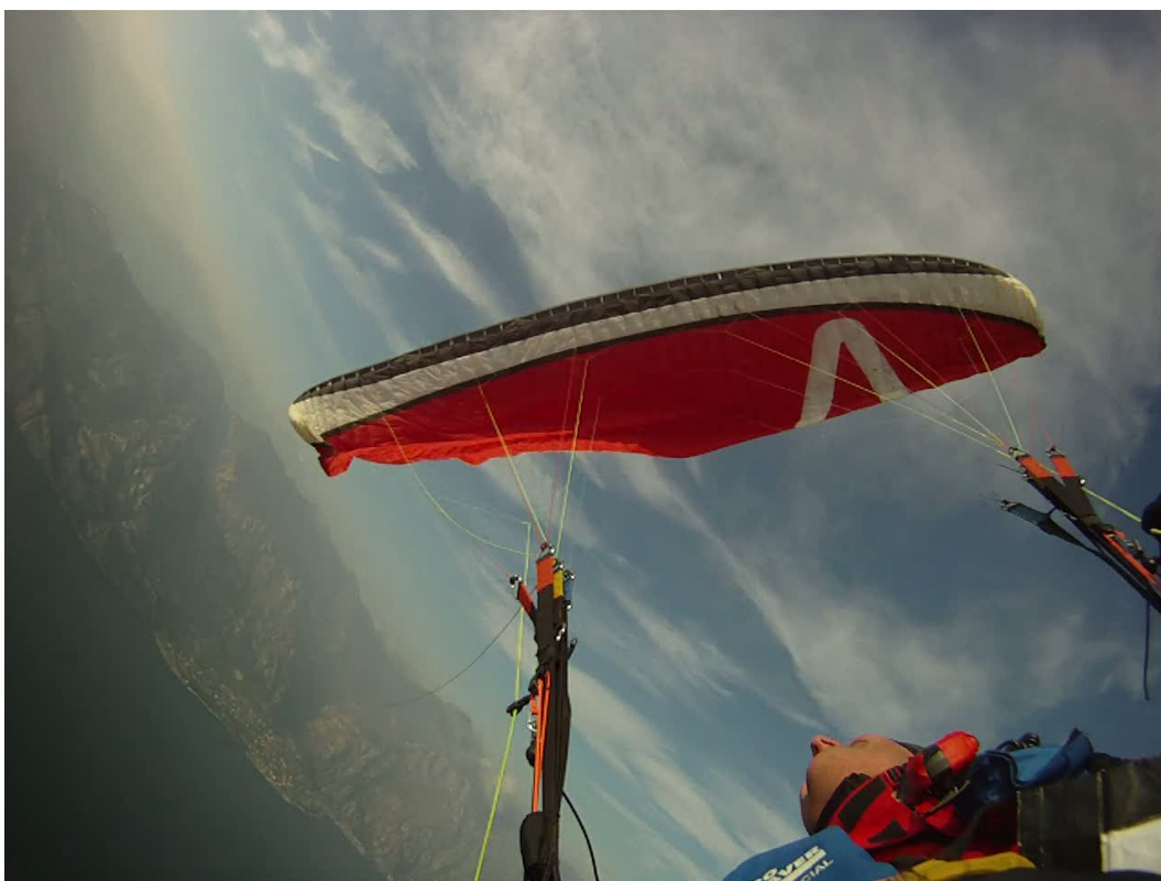
Picture 5: Active recovery required from test pilot to release cravat and stop the dive.
