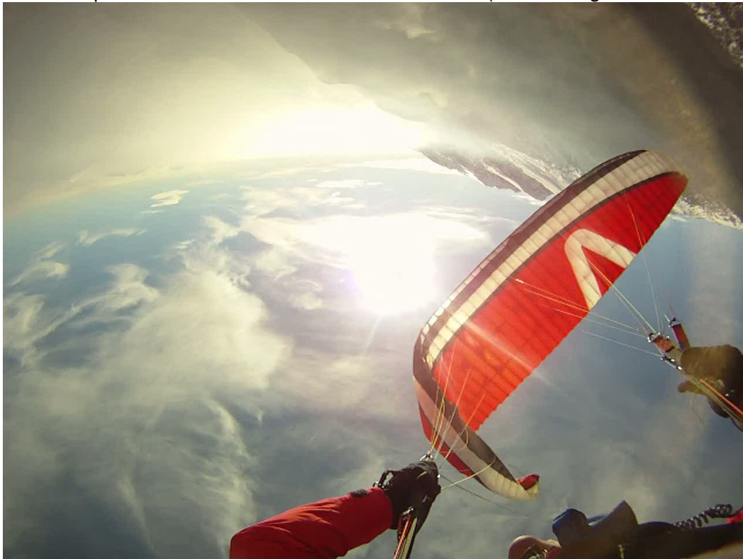
Picture 3: Outer wing tip collapse during wing-over manoeuvre.
